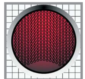
Rotary kiln chains
